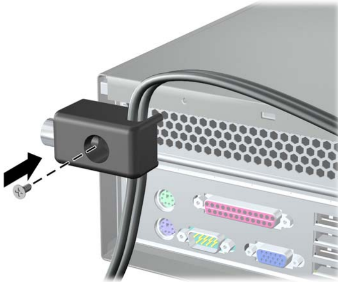
Figure 7-44 Attaching the Lock to the Chassis
